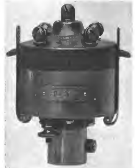
These two views of the Bosch timer-distributor show the very compact nature of the design and how access to the breaker is obtained by removing the distributor head
